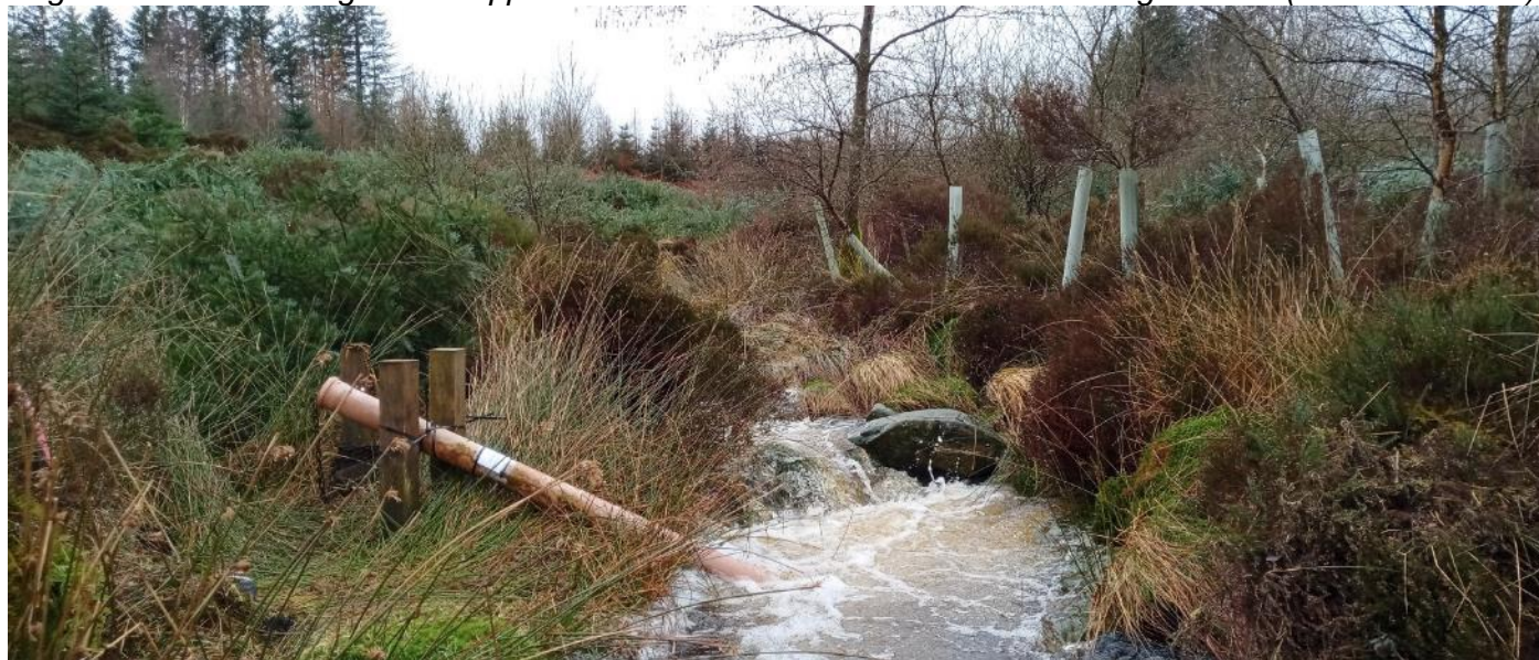
Figure 1 – Frame designed to support the EXO1 Sonde within the Cleuch of Eglon Burn (Fleet catchment)
